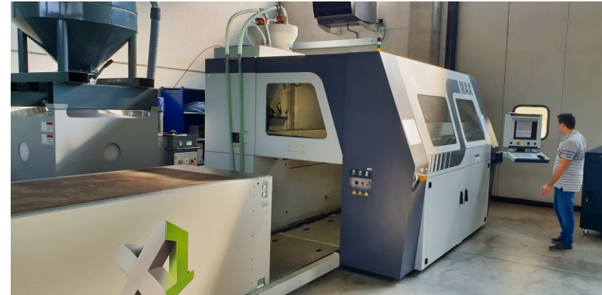
3D printed sand moulds and cores production by binder jetting
