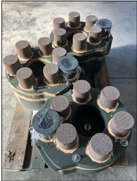
Moulds and cores assembled and ready for casting
