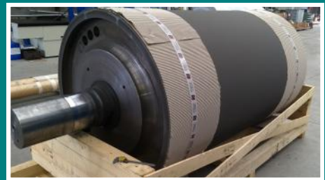
Continuous galvanizing line roll after coating
