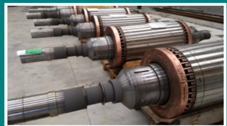
Electric rotors coated on the bearing seats and wear areas
