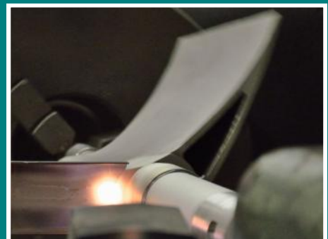
Coating of a guide vane
