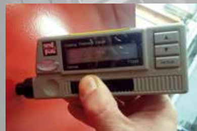
Controllo verniciatura Painting thickness
